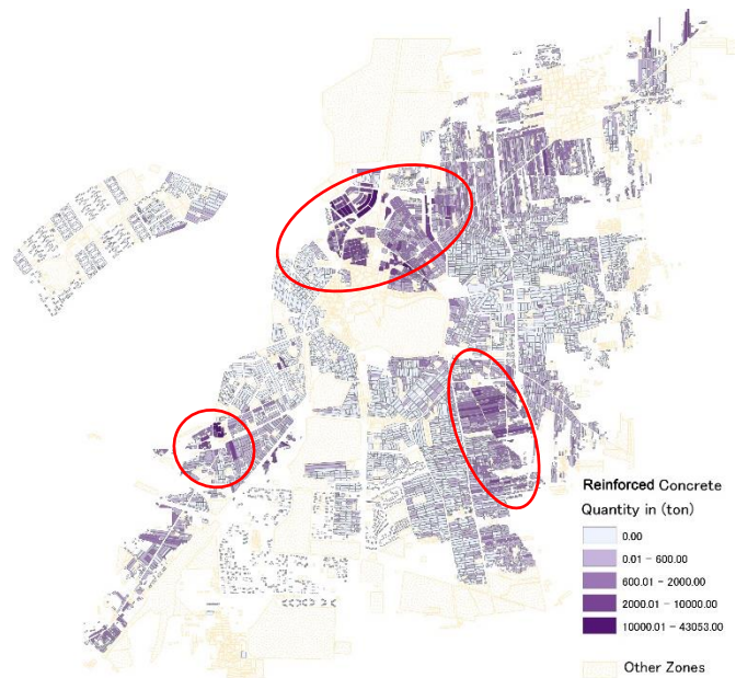
Figure 1. Distribution of damaged reinforced concrete in the residential buildings in Homs city. Red circles refer to the areas with high damage intensities.
