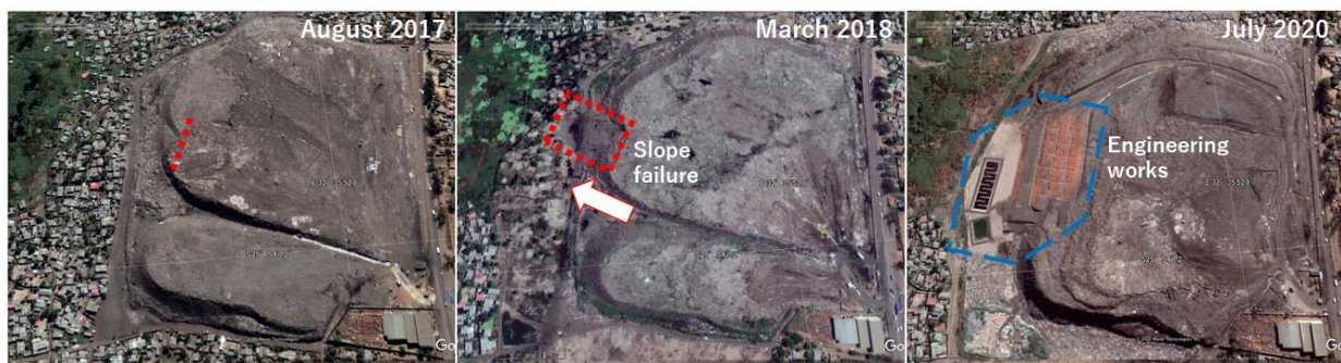
Figure - Landfill before (left) and 1 month after slope failure (center), and after rehabilitation (right)
